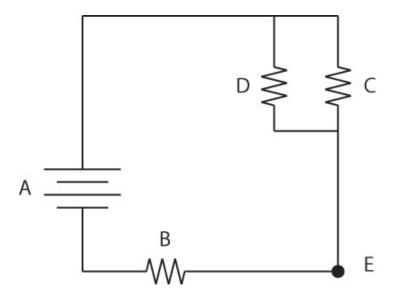
The voltage across A is 3 volts. The resistance of B is 1 ohm. The resistance of C is 3 ohms. The resistance of D is 4 ohms.
