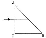
11. A prism whose angles are 45°, 45°, and 90° is illuminated by light entering as shown in the figure at right. To three significant figures, what is the minimum index of refraction the glass must have so that no light leaves the glass through the side AB?
