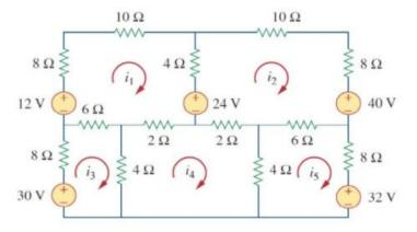
(a) Calculate the magnitude of current in loops  $i_1$ ,  $i_2$ ,  $i_3$ ,  $i_4$  and  $i_5$  in A. Round to 2 significant figures.
