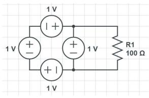
73. (3 points) Depending on its resistance, a component can have a voltage across it even if no current is flowing through it. Explain how an ideal voltmeter demonstrates this.
