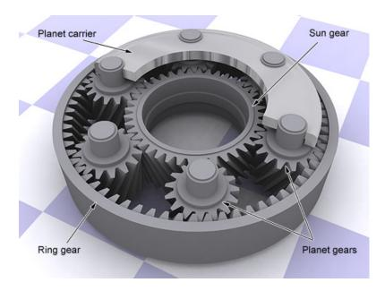
Calculate the ratio  $N_s/N_r$  of the number of teeth in the sun gear to the that of the ring gear in terms of  $\omega_s$ ,  $\omega_p$ ,  $\omega_c$ , and  $\omega_r$ , the angular velocities of the sun gear, planet gears, planet carrier, and ring gear respectively, positive clockwise.
