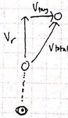
$$V_{\text{total}} = \sqrt{V_r^2 + V_{\text{tang}}^2}$$
