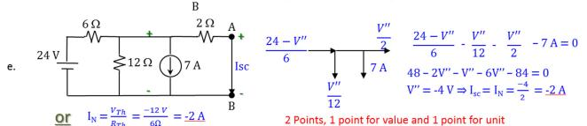
$R_N = R_{Th} = \underline{6} \Omega$  2 Points, 1 point for value, 1 Point for unit f.
