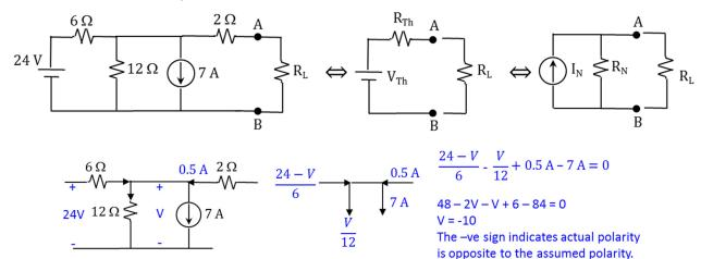
V = 10 =  $(R_L + 2) 0.5 \Rightarrow R_L = 18 \Omega$  2 Points, 1 point for value, 1 Point for unit
